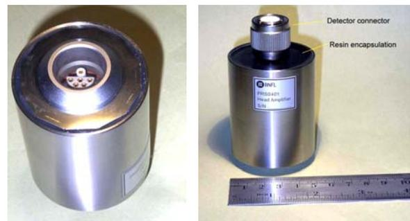
Figure 2: Head amplifier design showing the cable connection to the HUB unit
